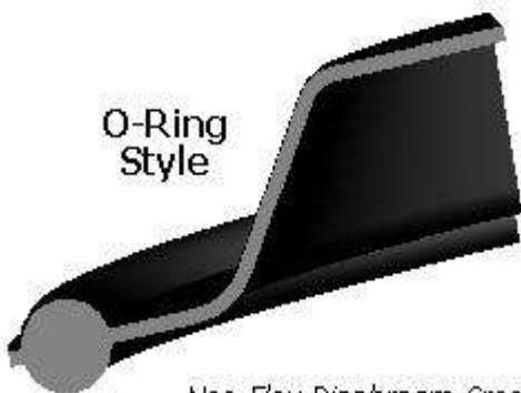
Neo-Flex Diaphragm Cross-Section
